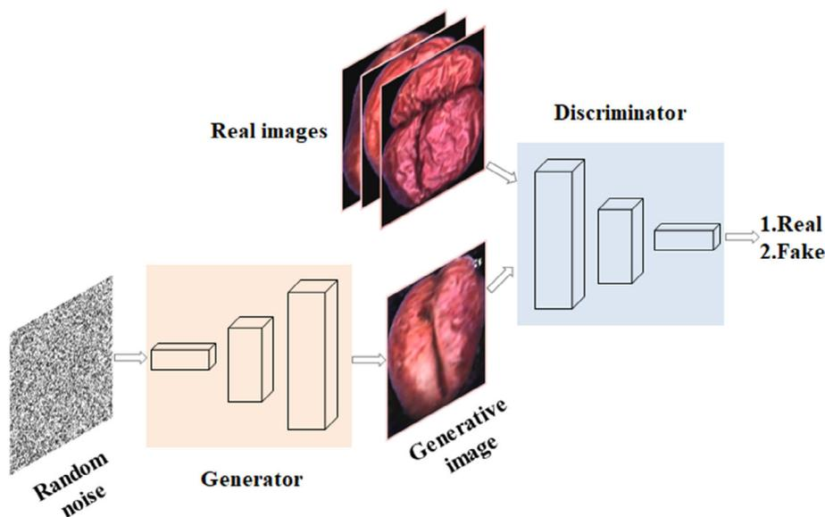
**FIGURE 7** The schematic diagram of deep convolutional generative adversarial network (DCGAN)
