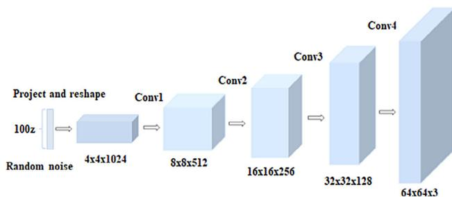
FIGURE 5 The structure of the generator
