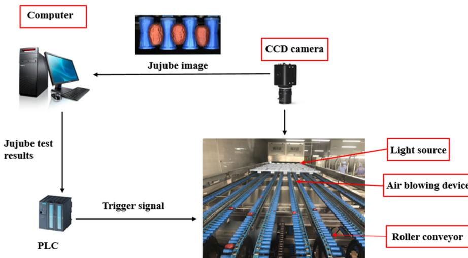
**FIGURE 1** Quality grading process of jujubes
