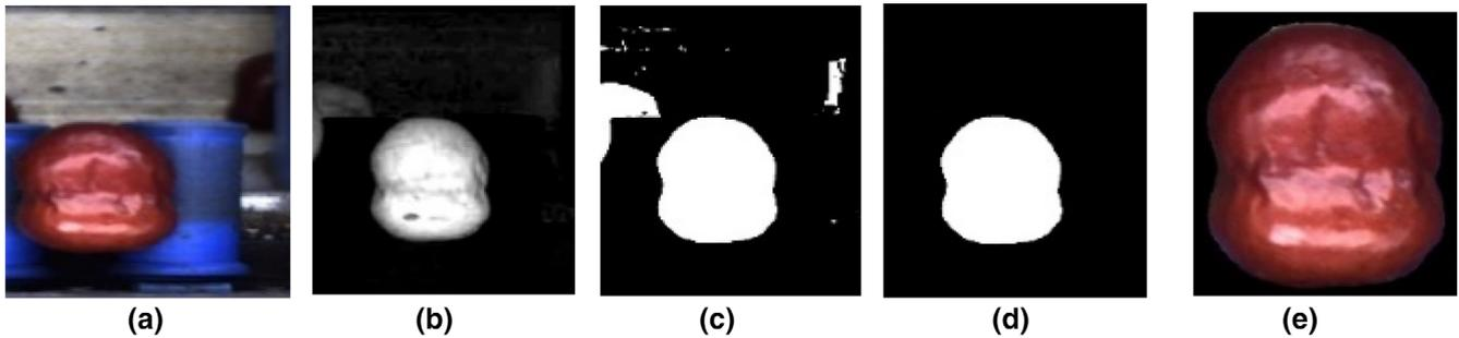
FIGURE 4 Jujube target extraction: (a) original image; (b) grayscale; (c) binarization; (d) denoising and extraction; (e) result
