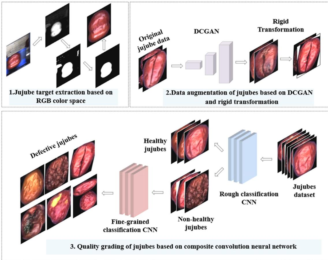
FIGURE 3 The schematic diagram of quality grading method of jujubes
