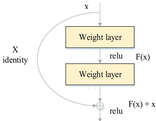
**FIGURE 8** A building block of ResNet18
